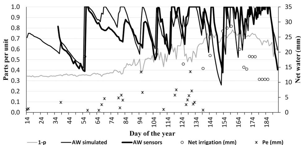
Fig. 7. Comparison between simulated (MOPECO) and measured (potential sensors) available soil moisture content progression in the ND treatment (2016). p: fraction of total available water that a crop can extract without suffering water stress (main Y-axis); AW: available water (main Y-axis); Pe: effective precipitation (secondary Y-axis); net irrigation (secondary Y-axis).
