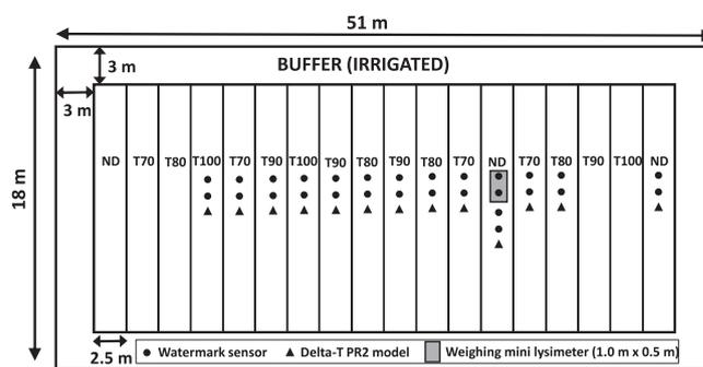
Fig. 3. Distribution of the different treatments in the experimental plot and location of the soil moisture sensors. Note: The weighing mini lysimeter was installed in the plot occupied in 2016. ND: No deficit treatment; T100, T90, T80 and T70: Treatments corresponding to 100% 90%, 80% and 70%, respectively, of garlic net irrigation requirements in the weather conditions of the intermediate typical meteorological year.
