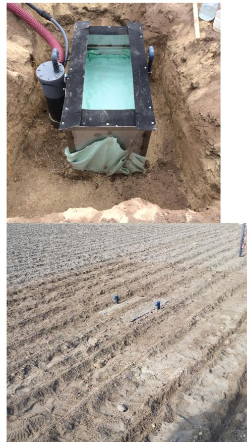
Fig. 4. Installation of the continuous weighing mini lysimeter.
